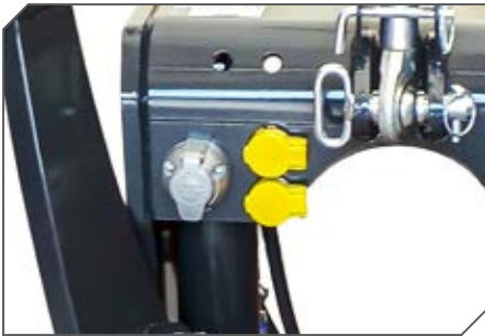
Double-acting front hydraulic connections (two hoses with quick couplings integrated on the cross-bracket).
