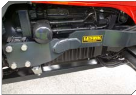
Support for gearbox housing (lateral mounting brackets extended to the gearbox housing).
