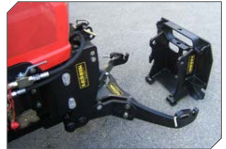
Snow plow mounting plate (for attaching a snow plow in the winter season).
