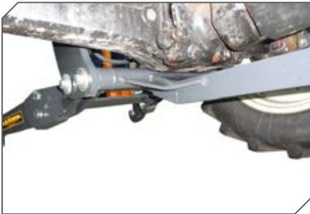
Extra reinforcement connecting the front linkage to the rear of the tractor. Essential for heavy duty applications.
