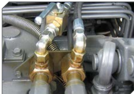
"T-joint" for the rear quick coupling of the tractor.
